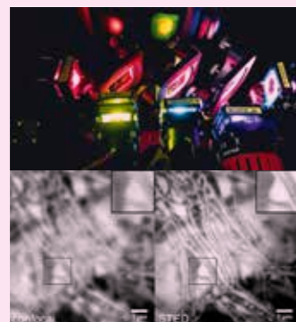
The group develops new optical imaging approaches and applies them to biological questions. Top: Close-up of an optics module in one of the group's super-resolution microscopes. Bottom: Nerve cell processes of living cultured neurons imaged with both super-resolution STED and conventional diffraction-limited (confocal) microscopy. STED reveals considerably more detail.
