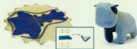
A self-transforming structure: fabricated as a flat object, once released it deforms into a predefined surface through a process controlled locally by the assemblage of small-scale structures.
